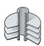
The keyfin is manufactured by forming a helical groove in the tube surface, winding the fin into the groove and peening the displaced metal from the groove against the fin. This means a tight fit between the fin and the tube. The keyfin is the superior design for dissimilar tube and fin material. Keyfin
